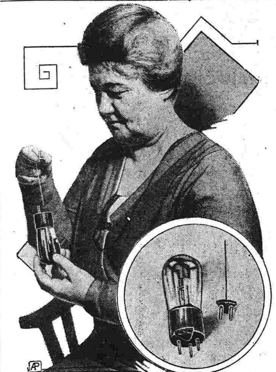
Mrs. Clara E. Quinn, electrical engineer of Cleveland, Ohio, demonstrating her newly developed radio tube with a replaceable filament. At the right is a closeup of the tube and "darning needle" filament.
